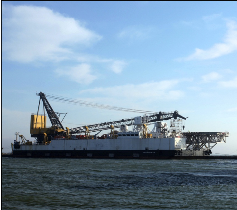
800 MT CRANE HAS BEEN FULLY INSTALLED
