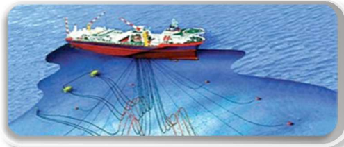
FPSO Mooring, Riser Installation and Hook-up
